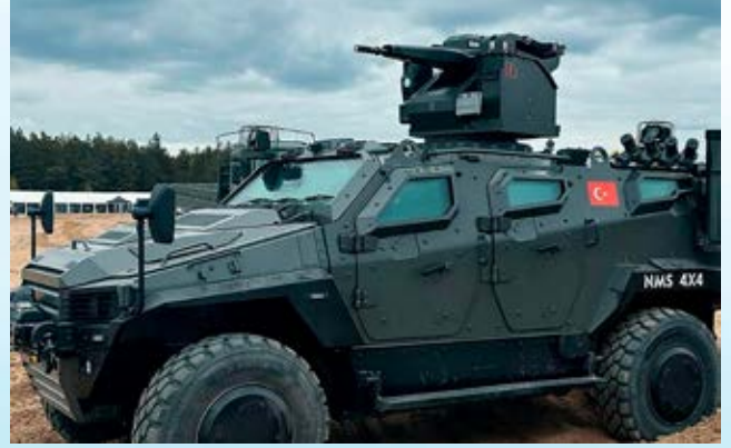
SYS Grup- UNIROBOTICS TRAKON 30 Uzaktan Komutalı Silah Sisteminin NUROL MAKİNA NMS 4X4 Aracına Entegrasyonu Integration of SYS Group-UNIROBOTICS TRAKON 30 Remote Controlled Weapon System into NUROL MAKİNA NMS 4X4 Vehicle
