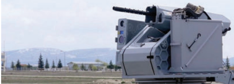
SYS Grup CANiK & UNIROBOTICS TRAKON 12.7 Remote-Controlled Weapon System, equipped with the 12.7 mm CANiK M3
