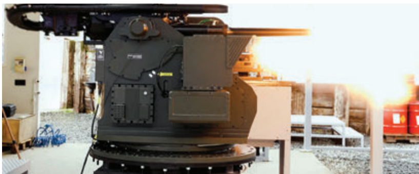
UNIROBOTICS 30x113 mm VENOM LR ile donatılmış TRAKON 30 Uzaktan Komutalı Silah Sistemi SYS Group- AEI Systems & UNIROBOTICS TRAKON 30 Remote Controlled Weapon System equipped with 30x113 mm VENOM LR
