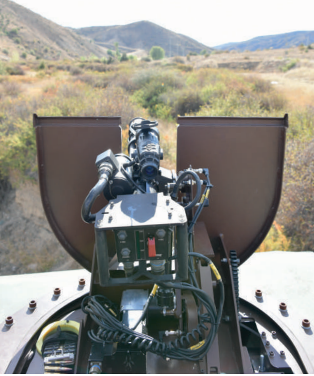
SRS, Unidef'in, uzaktan kumandalı ve platform içerisine katlanabilir silahlı taret (AAT) sistemi üzerinde şekillendirildi. ATS was based on Unidef's remote controlled gun turret (AAT), which can also be folded into the platform.
